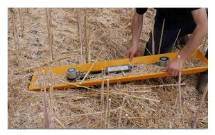
After sample has been collected from the rear of the harvester, the centre frame of the tray with magnets can be removed, ensure to include any grains on top. Separate the seeds from the chaff and either manually calculate or enter grain count or weight into the app for calculations.
