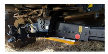
Connect tray via magnets to harvester, connecting the hood first followed by the tray. Ensure that the power has been turned on and the indicator is flashing green. DO NOT mount in front of wheels!
