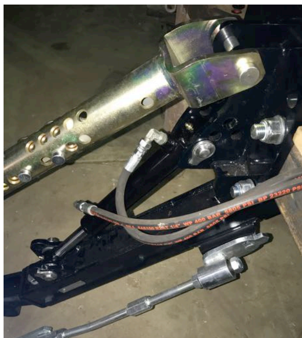
Image 3: 1.5" hydraulic ram and top link installed with suggested hose layout
