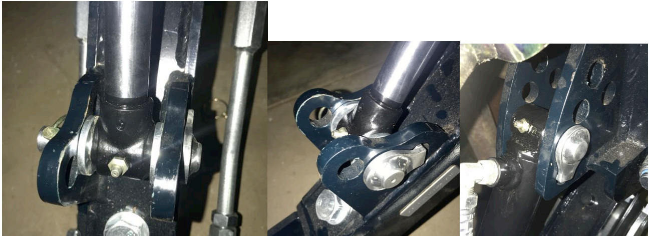
Image 2: 1.5" (2021 onwards) Ram installation
