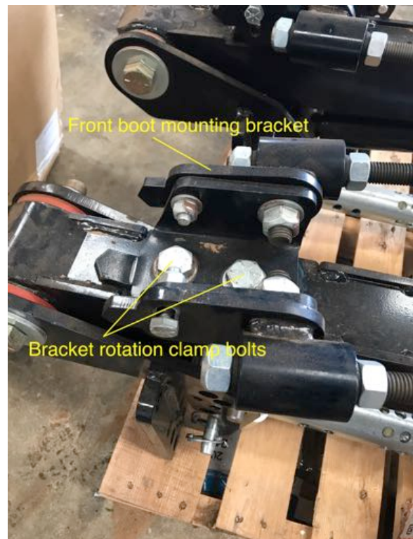
Image 5: Front seed boot mounting bracket
